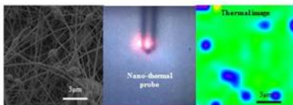
Scanning electron microscopy and transition temperature microscopy images of zein electrospun nanofibres
