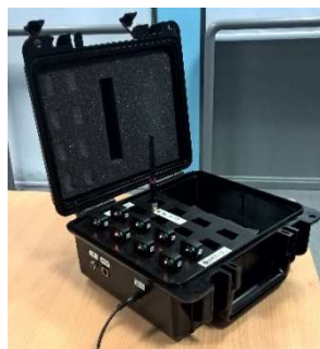
Figure 5.5. The Trigno (Delsys®, Boston, USA) wireless EMG system.
