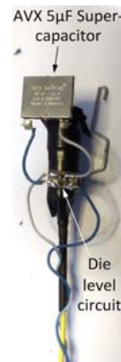
Figure 4. Rectification and storage circuitry.
