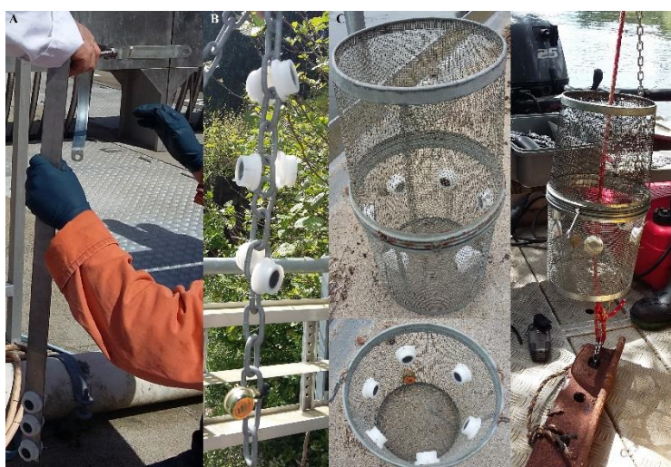
Figure 3.5 a) DGTs secured on a stainless steel bar b) DGTs secured on a galvanised steel chain c) DGTs secured in a galvanised steel cage.
