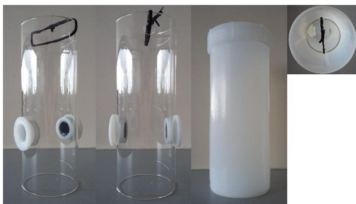
Figure 2.3 DGTs trial cell made up of silanized pyrex glass and hydrophobic perfluoroalkoxy alkane (PFA) container and screw cap.
