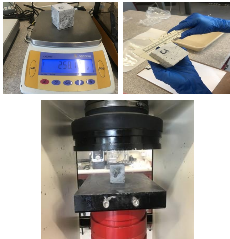
Figure 36: Measuring and compressive tests
