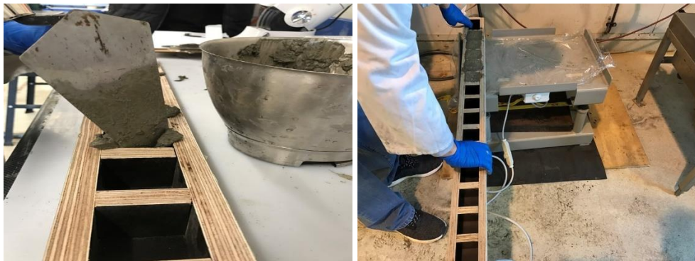
Figure 31: Casting and compaction of the samples
