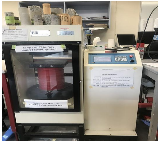
Figure 25: Images of compressive machine
