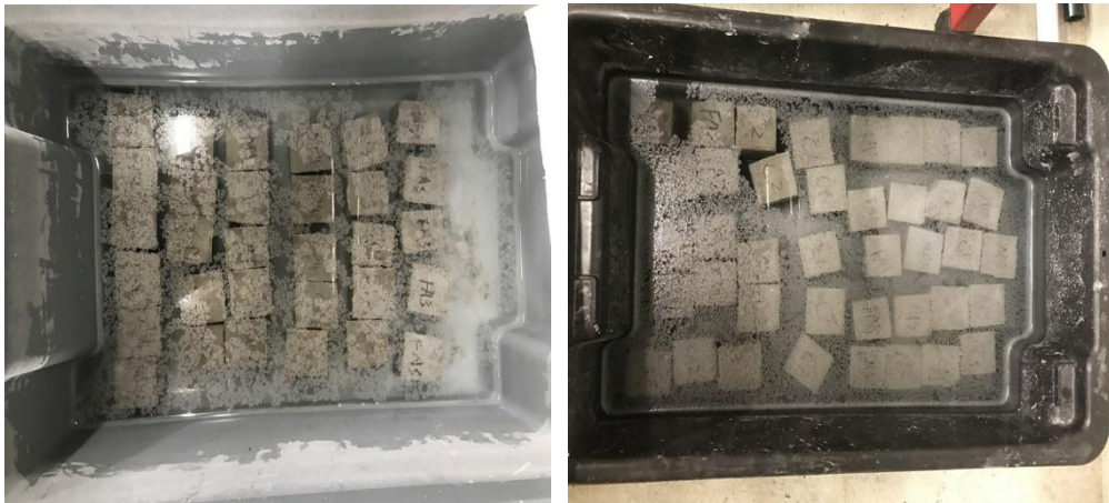
Figure 33: Water curing of the samples
