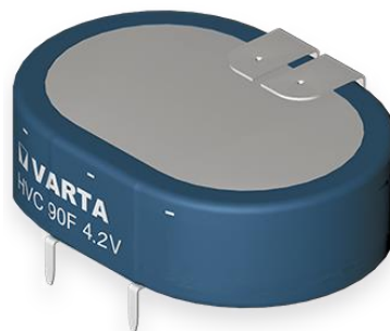
Figure 3.6. 90F, 4.2V hybrid supercapacitor.
