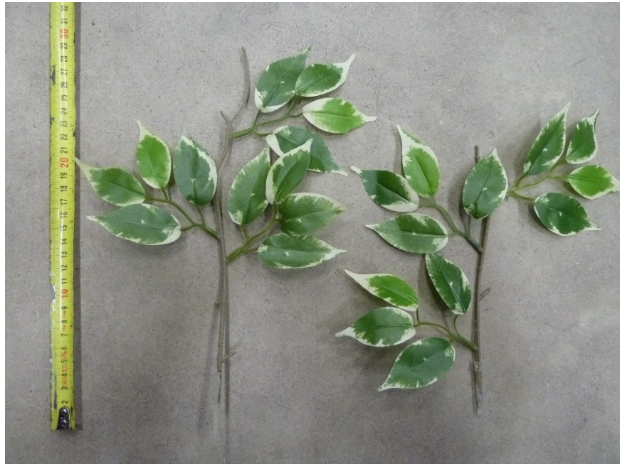
Figure 12: Artificial plants used in drag force measurements. Tall (left) and short (right) plants in their 3-leaf configurations. Both plants have their largest projected leaf area facing towards the camera.
