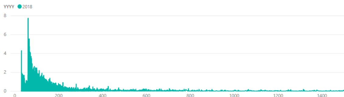
Figure 20: Volume of intraday trading in GWh as a function of minutes before the delivery of energy in Finland in 2018 (Fingrid 2019h).
