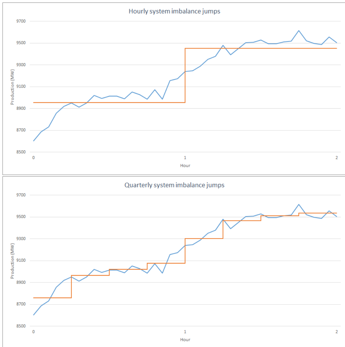
Figure 18: In both graphs, the blue line represents actual production in Finland between 07:00 – 09:00 in the morning of January 16, 2019. In the upper graph, the orange line represents hourly scheduled production positions, whereas in the lower graph the orange line represents quarterly scheduled production positions.
