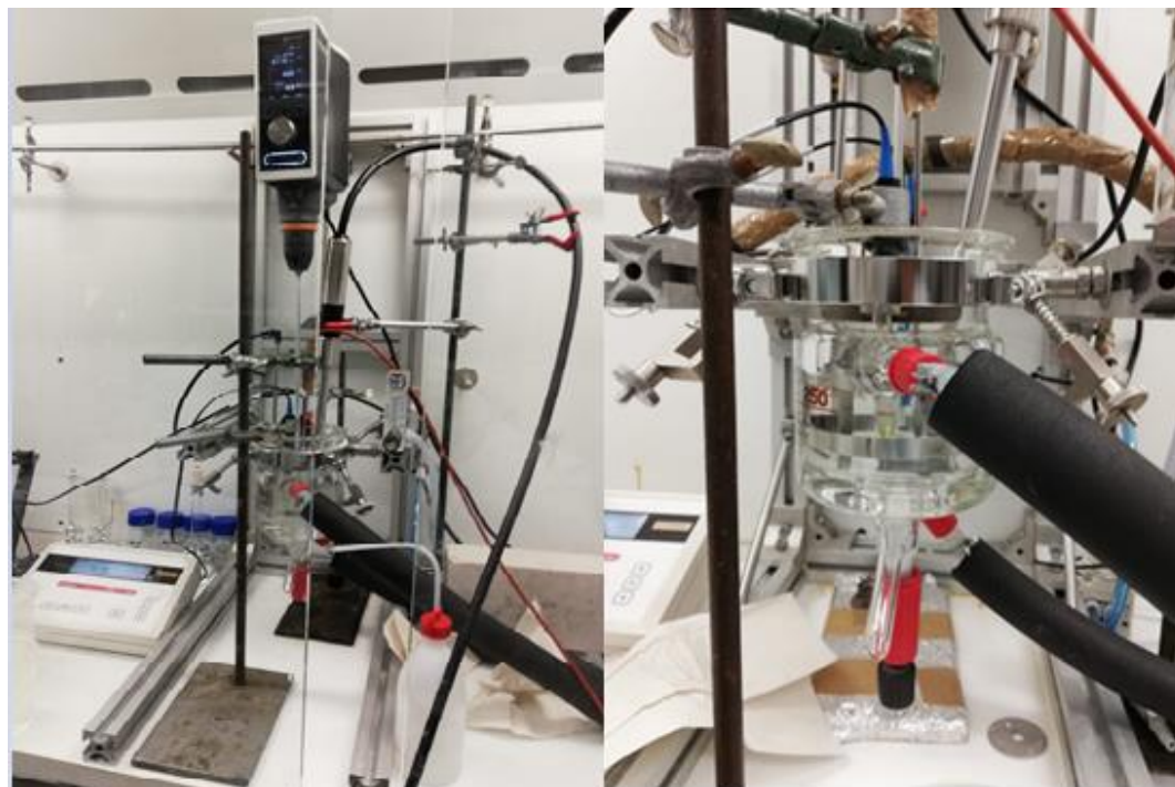
Figure 22. Experimental setup of lithium carbonate precipitation in heterogeneous system.
