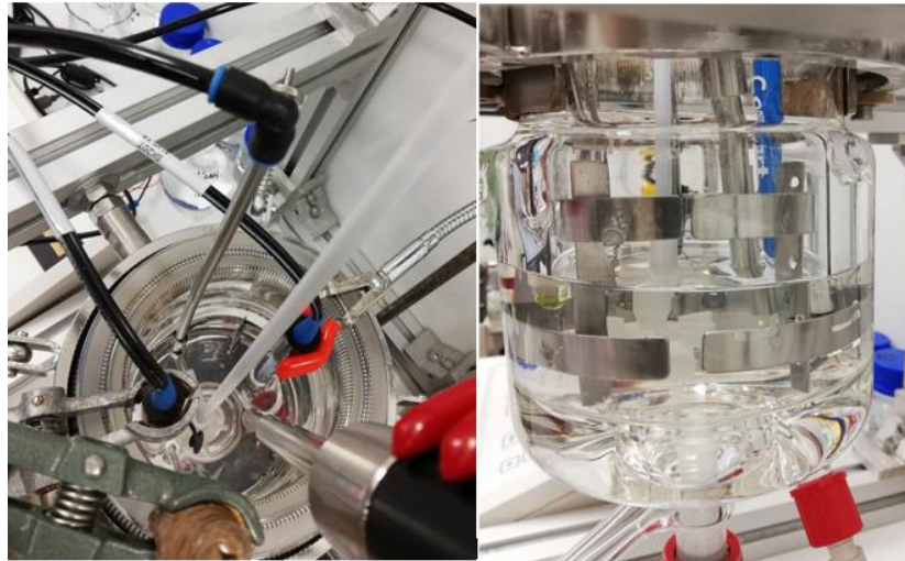
Figure 29. Close-up of the continuous stirred tank reactor used in the experiment.
