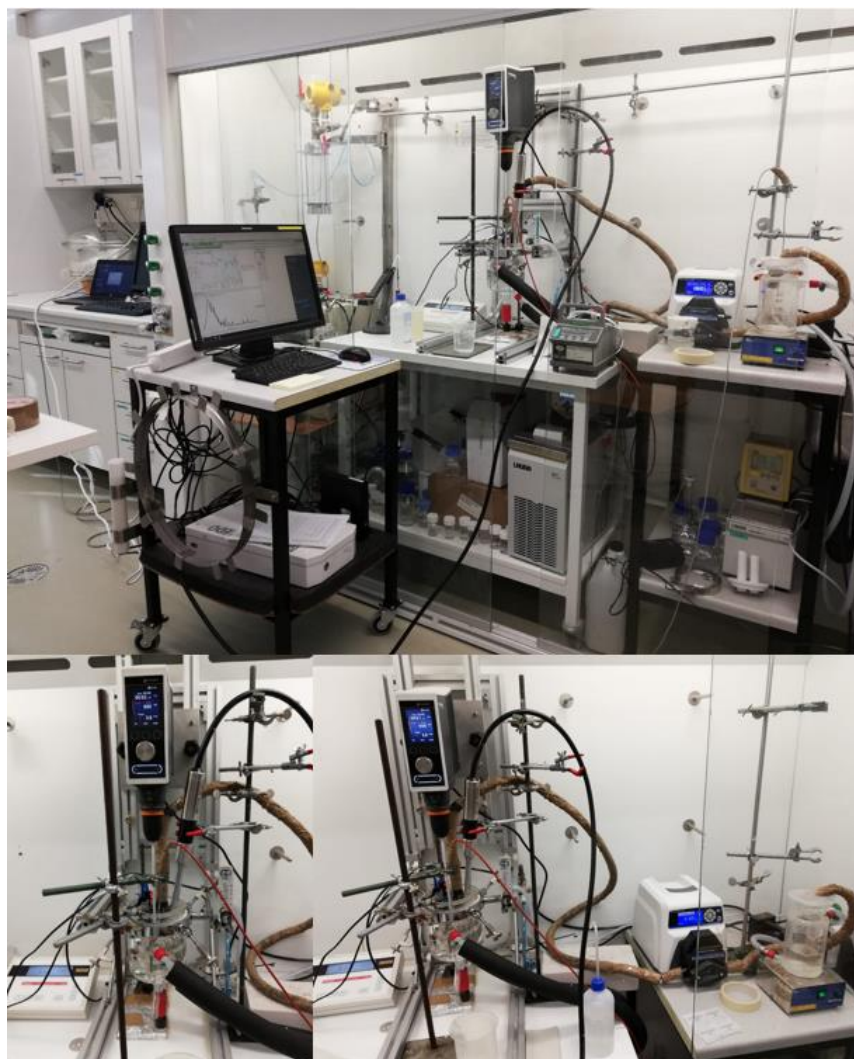
Figure 28. Experimental setup of lithium carbonate homogeneous reactive crystallization system. The crystal yield and filter cake moisture were determined in a similar manner as described in section 10.3.1.
