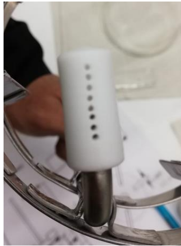
Figure 17. Sparger used in this study.
