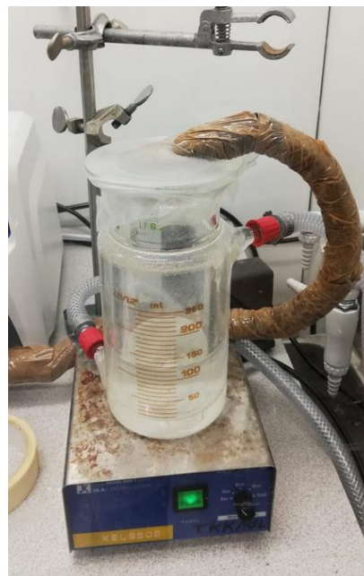
Figure 30. Close-up of the sodium carbonate dissolution vessel.
