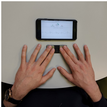
Figure 1: ECG monitor connected to the smartphone application.
