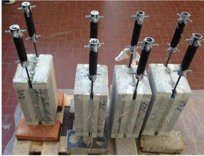
Figure 8. Installation of steel pipes on the ends of the carbon FRP bars
