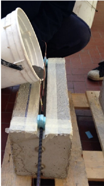
Figure 5a. Cast of cementitious mortar in the groove
