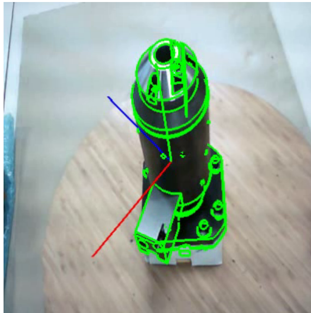
Figure 4.10: Recognition example of a real industrial object (see Fig. 4.1). Note how the projection of the model edges (green) perfectly aligns with the object in the image.
