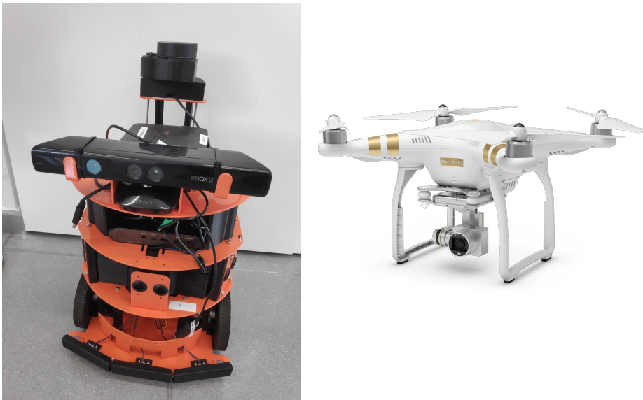
Figure 1.4: Left: an autonomous mobile robot equipped with an RGB-D camera and a laser scan. Right: an autonomous flying drone equipped with an RGB camera ©DJI.
