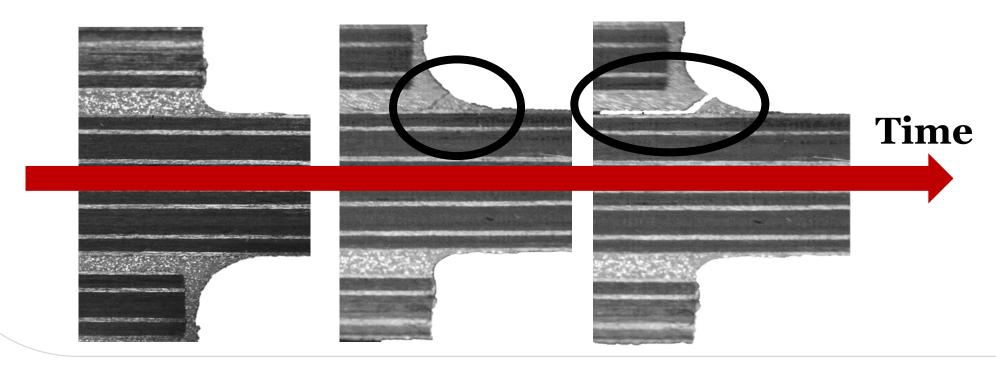
**High Speed Camera** used to capture failure mechanism for **36mm overlap length**
