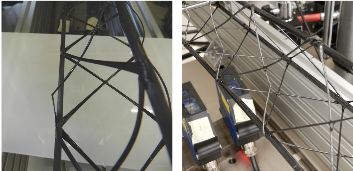
Figure 14: Failure in large section truss configurations: a) L-F; b) L-T.
