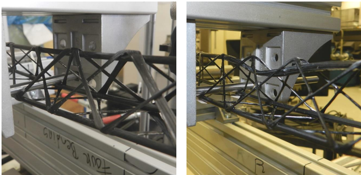
Figure 15: Failure in small section truss configurations: a) S-F: debonding; b) S-T: debonding and chord failure.
