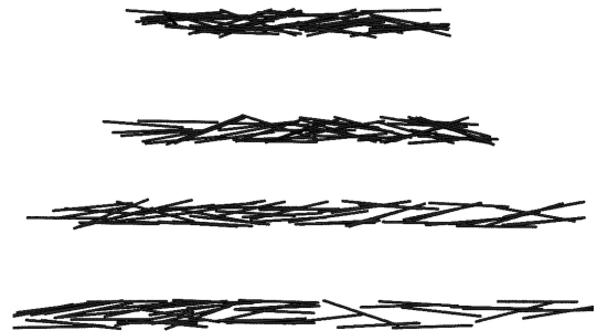
Fig. 9. Fibre alignment for plate spacings of 1.0mm for jet velocities of 0.4m/s, 0.8m/s, 1.6m/s, 3.2m/s (top to bottom)
