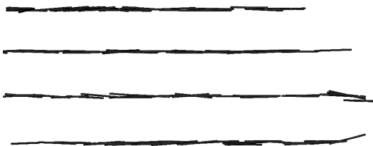
Fig. 8. Fibre alignment for plate spacings of 0.3mm for jet velocities of 0.4m/s, 0.8m/s, 1.6m/s, 3.2m/s (top to bottom)
