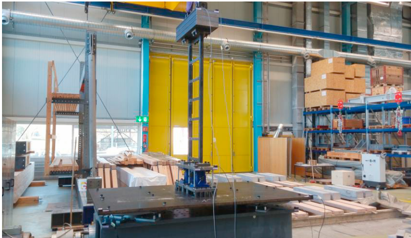
Fig. 2. Experimental setup of the cantilever base-isolated structure in ETH Structural Testing Laboratory
