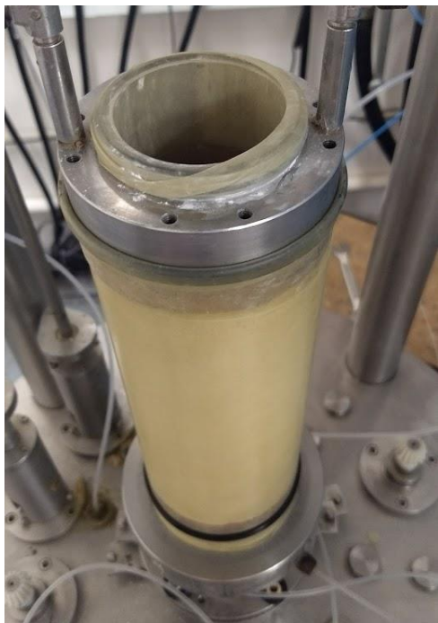
Figure 3. Image of prepared hollow cylindrical sample.
