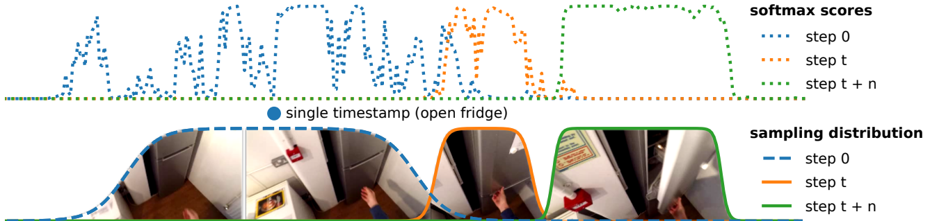
Figure 4. Updating the sampling distribution using the classifier response - example from action ‘open fridge’ in EPIC Kitchens [8]. Different colours indicate different training iterations.
