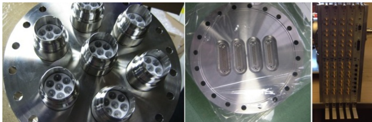
Figure 8.3.7: Photographs of the PMT HV flange (left), the 32-channel PMT signal flange (middle) and a 32-channel crate that mounts on the signal flange.
