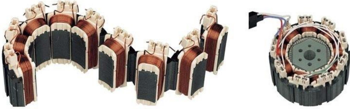
Figure 1. 14: Modular structure of POKI-POKI™ machine [32]
