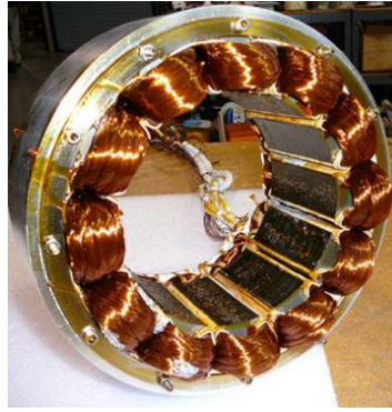
Figure 2. 2: An example of double layer concentrated winding [64]
