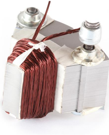
Figure 2. 35: An example of one segment of the 11kW high speed PMSM [86]
