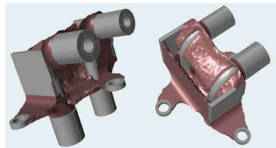
Figure 1: Optimized part obtained with Inspire
