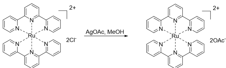
Figure 60. Synthetic scheme for model bis(terpyridine) metal complexes with acetate counterions for use in ITC experiments.
