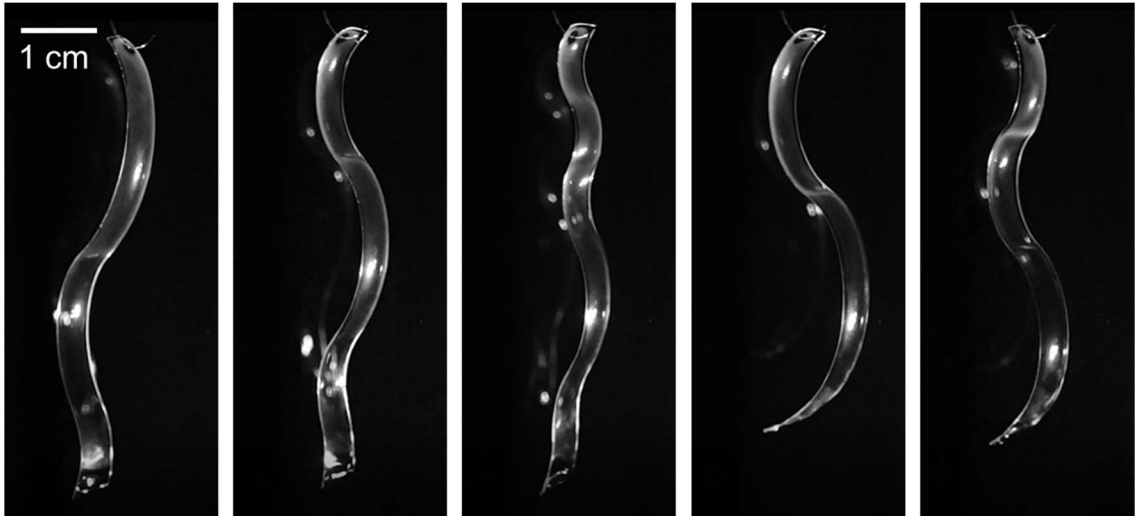
Figure 0.45 Various deformed shapes of a free-deswelling PDMS strip. A PDMS strip ( h_0 \sim 0.2 mm w_0 \sim 5 mm, L_0 \sim 50 mm) initially swollen with n-hexane was placed in a desiccator with one end connected to the lid by wire
