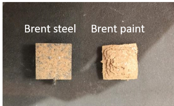
Fig. 5.31: Left: steel substrate with Shell coating gently peeled-off after immersion in N-methyl pyrrolidone. Right: Peeled off paint from the painted steel sample.
