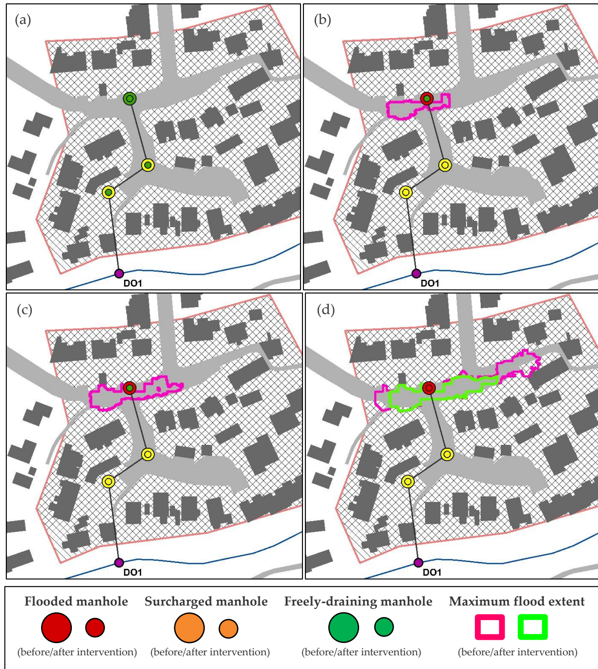
Figure 6: Functionality of Bridport surface drainage before and after upstream NFM interventions during a (a) 1 in 10 year storm; (b) 1 in 15 year storm; (c) 1 in 20 year storm; (d) 1 in 33 year storm
