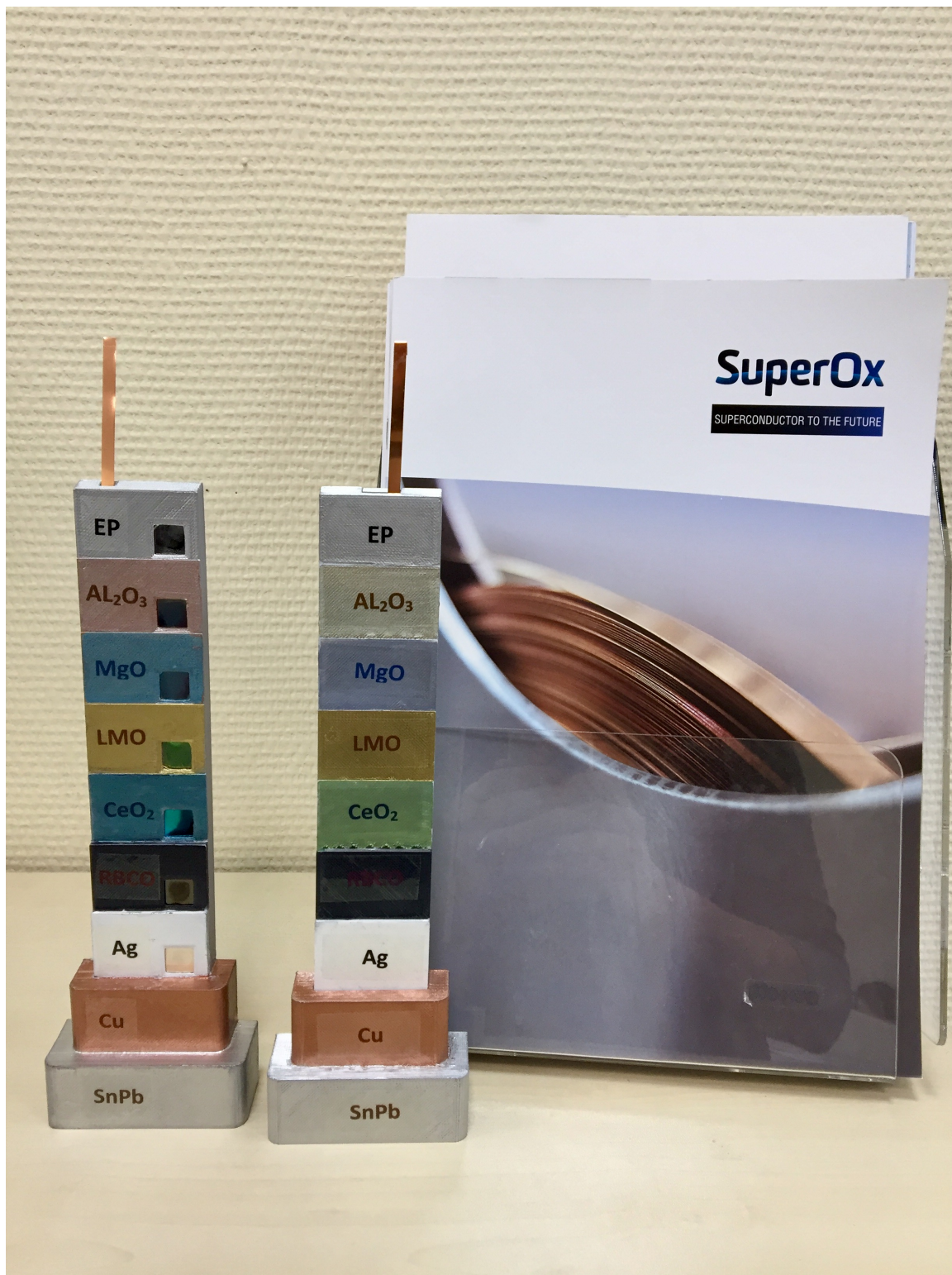
Figure 3 Photograph of Layers of Different Materials of SuperOx Superconducting Cable from Inside
