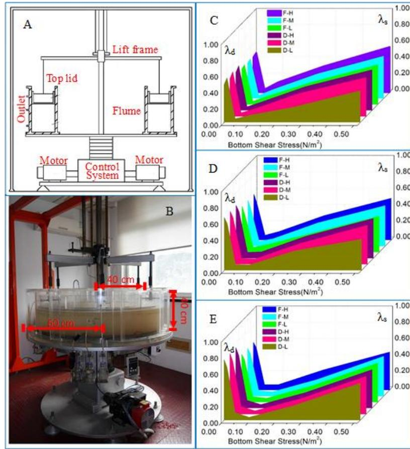
**Fig. 2.** (A) and (B) are, respectively, the schematic diagram and live photograph of the annular flume. (D), (E) and (F) are, respectively, the deposition and resuspension rates of Cu associated with fine, medium, and coarse-silt under varied shear stress.
