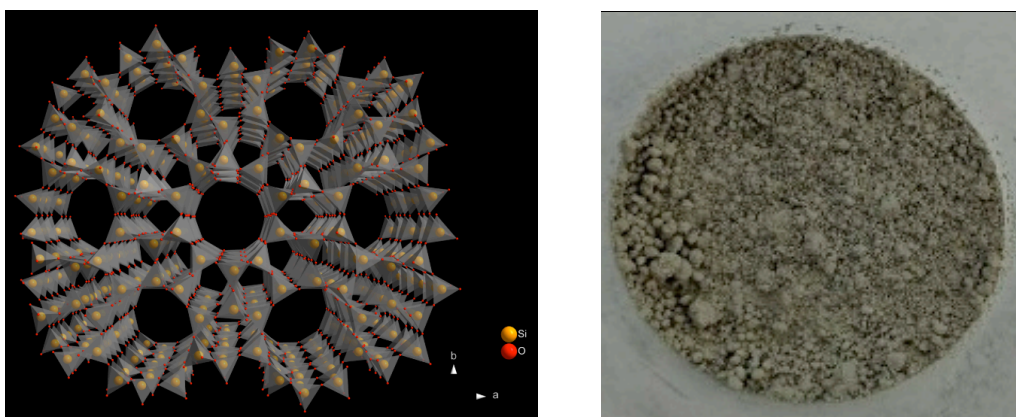
Figure 3-1 Zeolite ZSM-5 (a) a schematic of its structure and (b) a photograph showing the appearance of ZSM-5.
