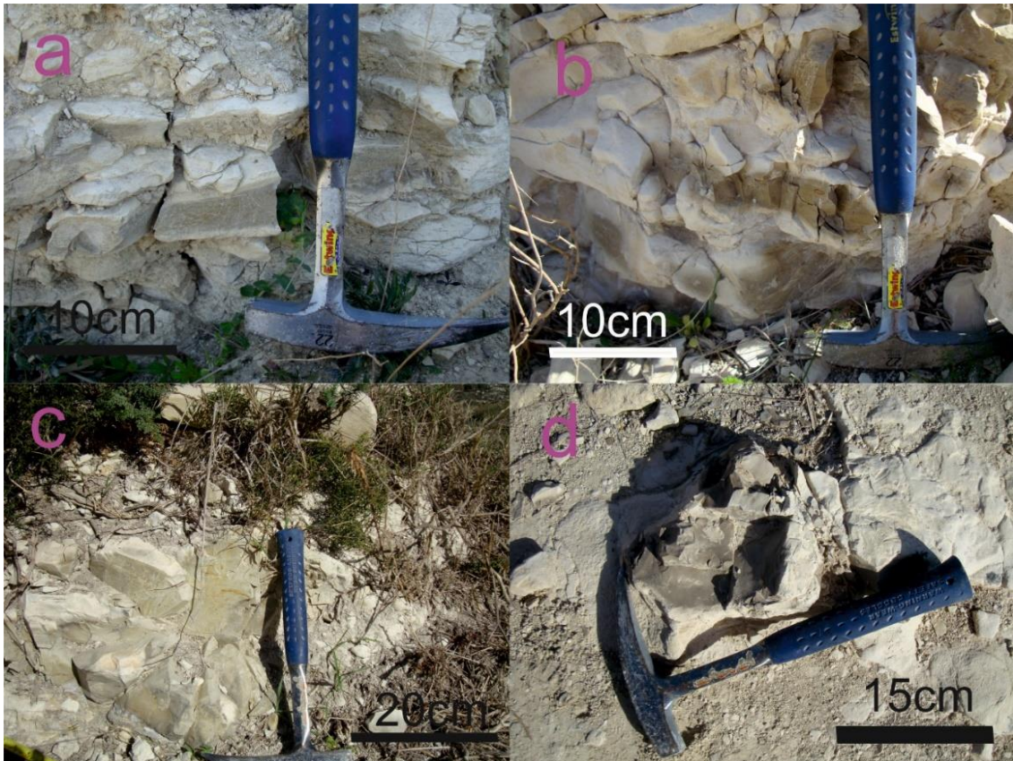
Figure 5-4: a) Bedded chert outcrops intercalated in bedded middle Globigerina Limestone, b) nodular chert with irregular shapes, c) Great exposure of chert outcrops and d) Nodular chert.
