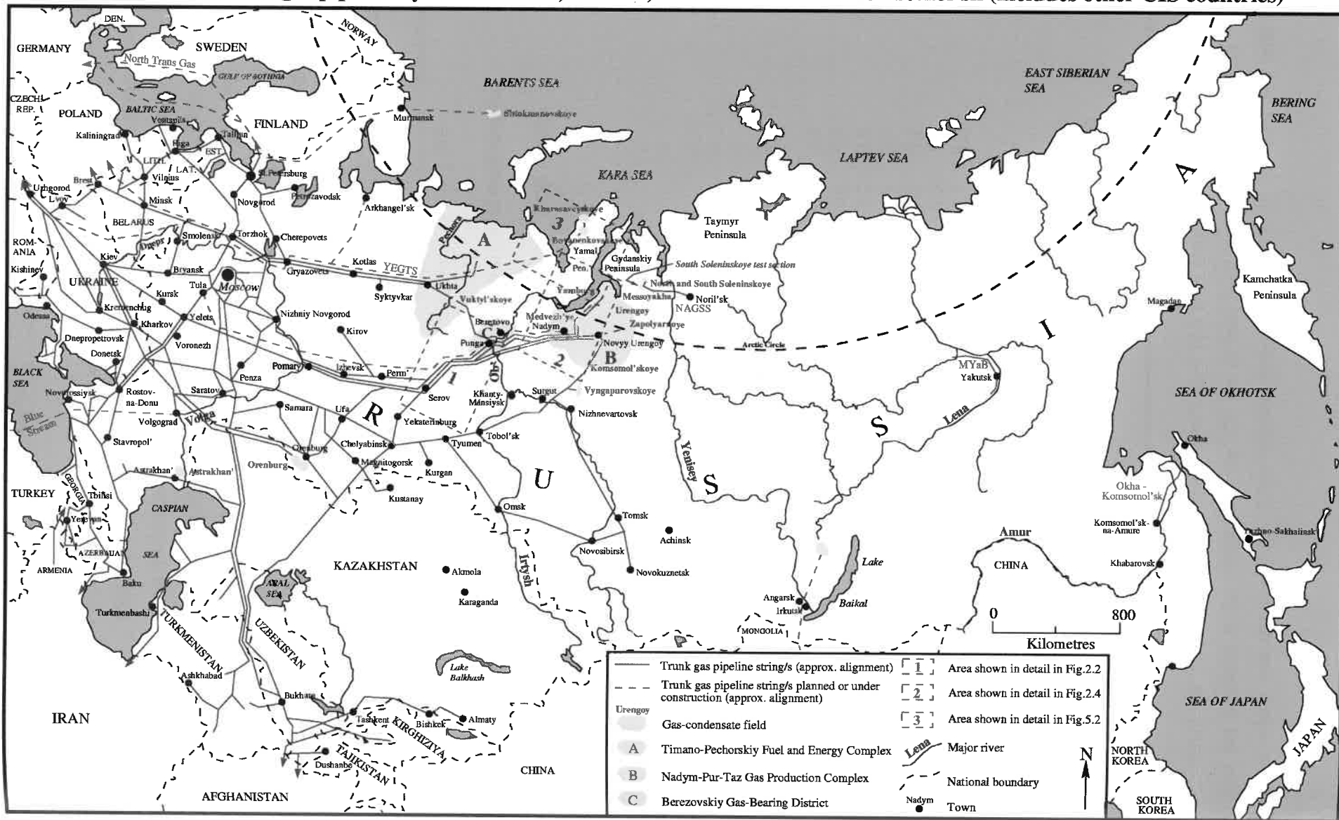
Fig.2.1 Russia's trunk gas pipeline systems : UGSS, NAGSS, MYaB and Okha - Komsomol'sk (includes other CIS countries)
