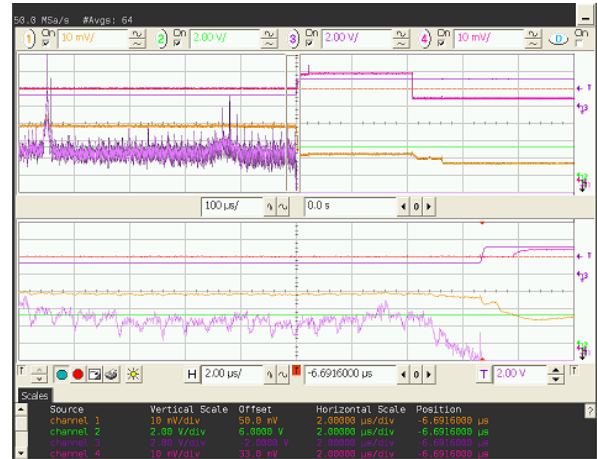
Fig. 8. Difference in power traces for corrupted bitstream.
