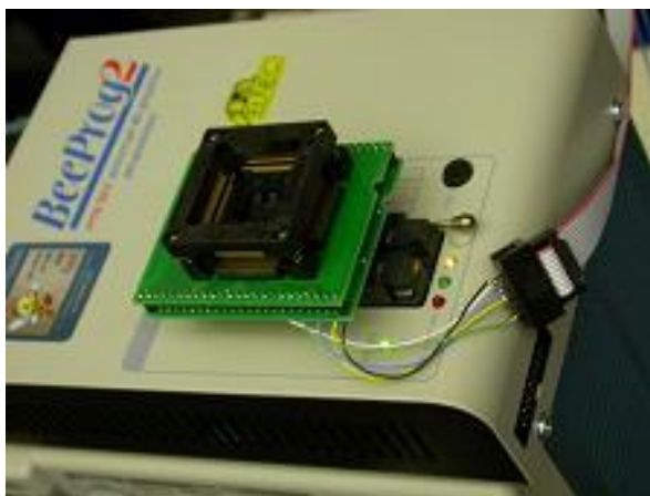
Fig. 2. Elnec BeeProg2 with modified PLD-18 adapter.
