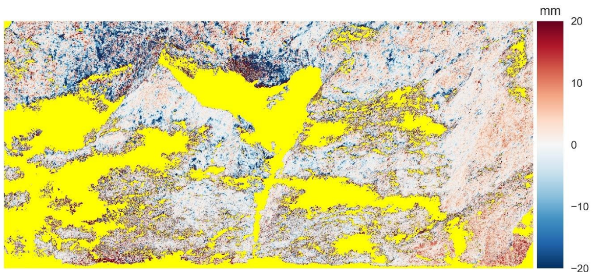
Figure 5.8. Difference of error DSM of the original image set compared with that with additive noise of 21 dB for the Overstrand site. Blue regions are those where the original set performs better in terms of error. No spatial trend was seen in terms of error with noise. No data (missing) values are in yellow.
