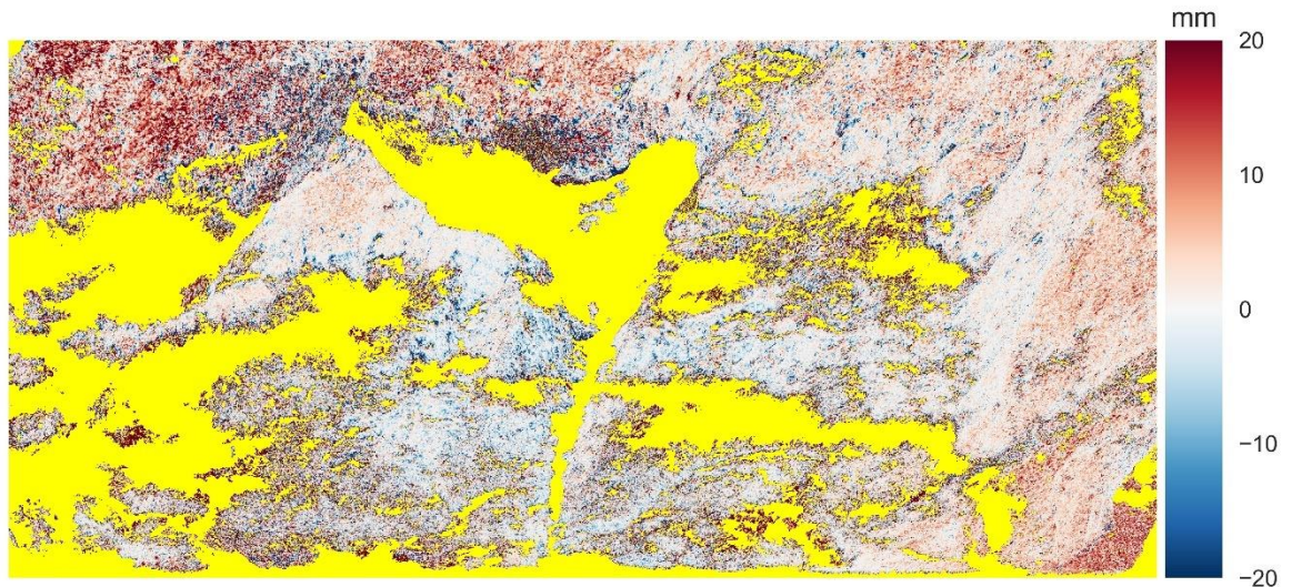
Figure 5.4. Difference of error DSM for the cloud produced from images compressed to ‘quality’ 92 compared with ‘quality’ 50 for the Overstrand site. Blue areas are where the more heavily compressed block is underperforming relative to the less compressed block. Higher levels of compression produced better results in terms of accuracy for occupied pixels. No data (missing) values are in yellow.
