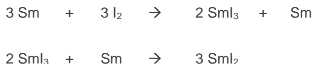
Figure 51. Imamoto's method to prepare \text{SmI}_2 , using samarium metal and iodine. 157
