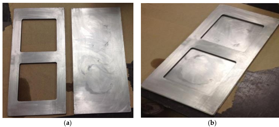
Figure 4. (a) Two-separate piece mold made of stainless steel; (b) Combined molds one serves as a window frame and the second as a baseplate.
