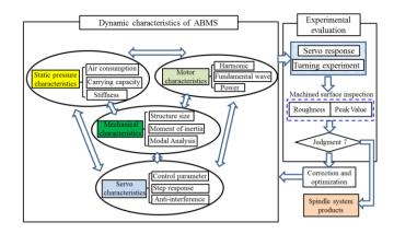
Fig. 2 Diagram of the electromechanical coupling approach
