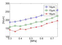
Fig. 9 Bearing stiffness versus air pressure
