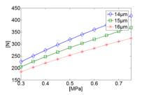
Fig. 8 Bearing capacity versus air pressure
