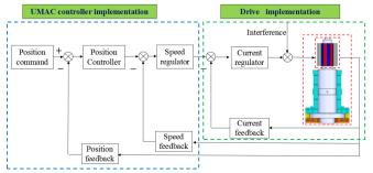
Fig. 17 Servo loop charts of the spindle system suppresses the speed fluctuations.<sup>26, 27</sup> The position loop ensures
