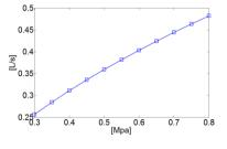
Fig. 10 Air consumption with air pressure
