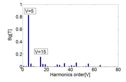
Fig.16 Space harmonics of the flux density
