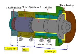
Fig. 1 Schematic diagram of ABS
