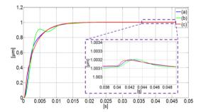
Fig. 18 Step response and anti-interference ability of ABS
