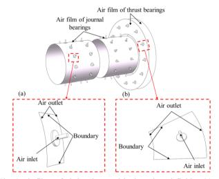
Fig. 4 Air films of air bearings and its boundary definition:(a) An orifice of journal bearings, (b) An orifice of thrust bearings
