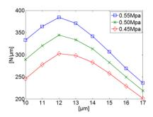
Fig. 7 Stiffness variation with film thickness
