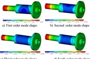
c) Third order mode shape d) Forth order mode shape Fig. 13 Mode shapes of the spindle shaft
