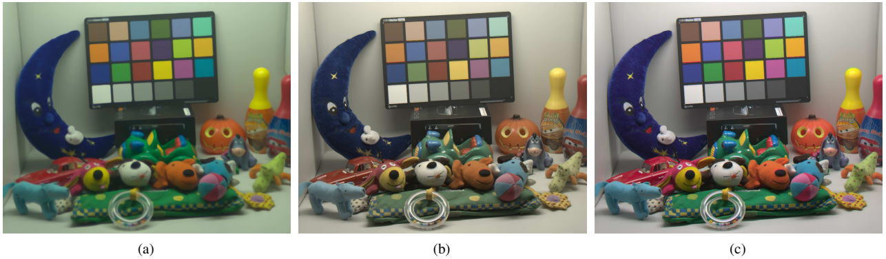
Figure 2: In (a), tristimulus values captured by the 2D Color Analyzer under the D65 illuminant, in cd/m^2 , converted into the sRGB color space and gamma corrected. In (b) an HDR photograph of the same scene. In (c), the HDR image has been color balanced, taking advantage of the color checker depicted in the image. The color balancing has been performed using the HDR Shop built-in method [hdr]. In both (b) and (c) the depicted colors do not match the ground truth acquisition.
