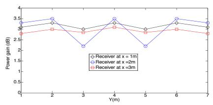
Fig. 4: Received optical power gain when the mobile user was walking along the y-axis and at x = 1 m, x = 2 m and x = 3 m in room B.
