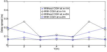
Fig. 3: Delay spread of the mobile user without and with the CGH in room A along x = 1 m and x = 2 m.
