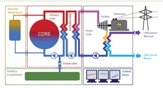
Fig. 2 SM-MS-R the modular concept. 1st module/container: core, primary and secondary. 2nd module/container: ternary, turbine/generator and cooling loop. 3rd module/container: waste management unit. 4th module/container: containment/accident MS catcher. 5th module/container: control room.
