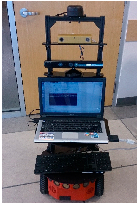
Figure 5. Pioneer P3-DX mobile robot with mounted sensors.
