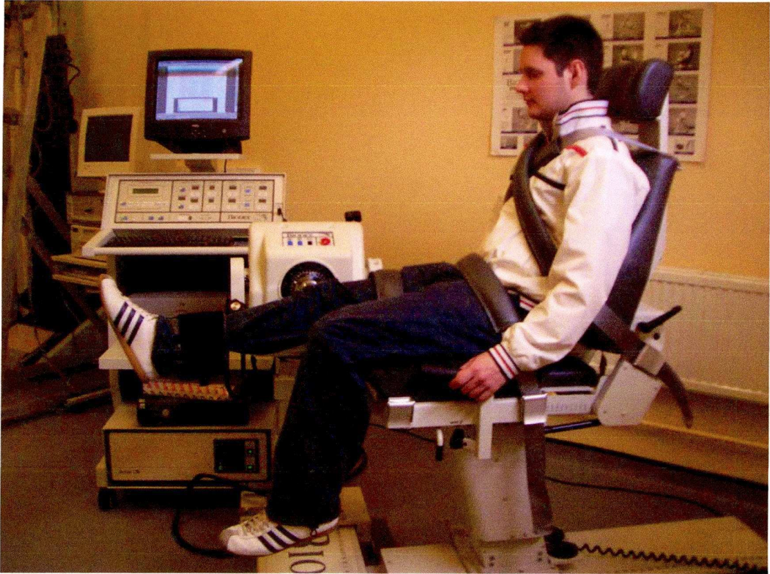
Figure 2.4: Lower limb peak skeletal muscle torque measurement using a Biodex Isokinetic dynamometer (published with subjects permission)
