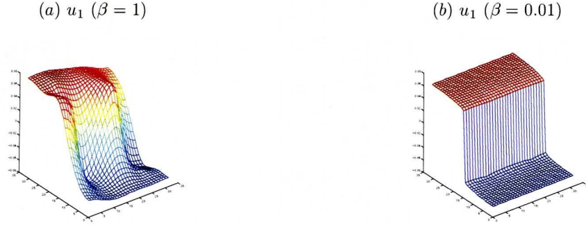
Figure 7.5: Surface plots of u_1 for the non-smooth registration problem shown in Figure 7.1 (a)-(b) (Example 1): results by \mathcal{R}^{\text{NewCv}} with (a) \beta = 1 and (b) \beta = 0.01 . (a) and (b) show smoothing effects on the surface of u_1 at two different values of \beta .
