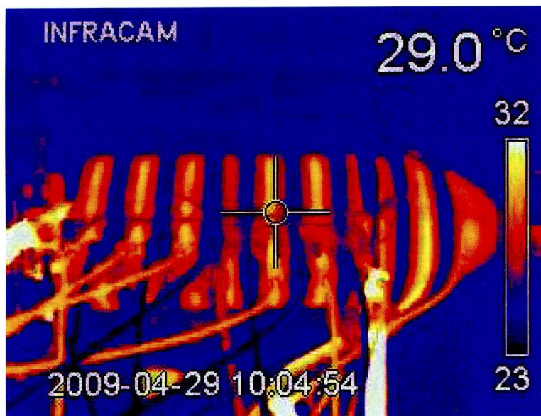
Figure C.3: Infrared camera picture showing the effect of water cooling on the main and upstream coils. 600 A current was used through the coils. Temperature scale is shown in the vertical bar on the right.
