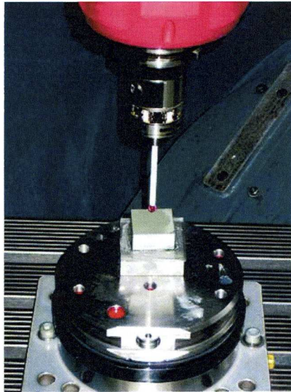
Figure 2: Infrared sensor (Renishaw OMP400)
