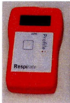
Figure 1-2: The Respirate, a respiration rate measuring device adopted as a respiration gating device.
