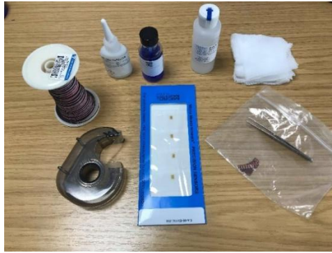
Figure 20 Accessories for installation of \mu -strain gauge sensor
