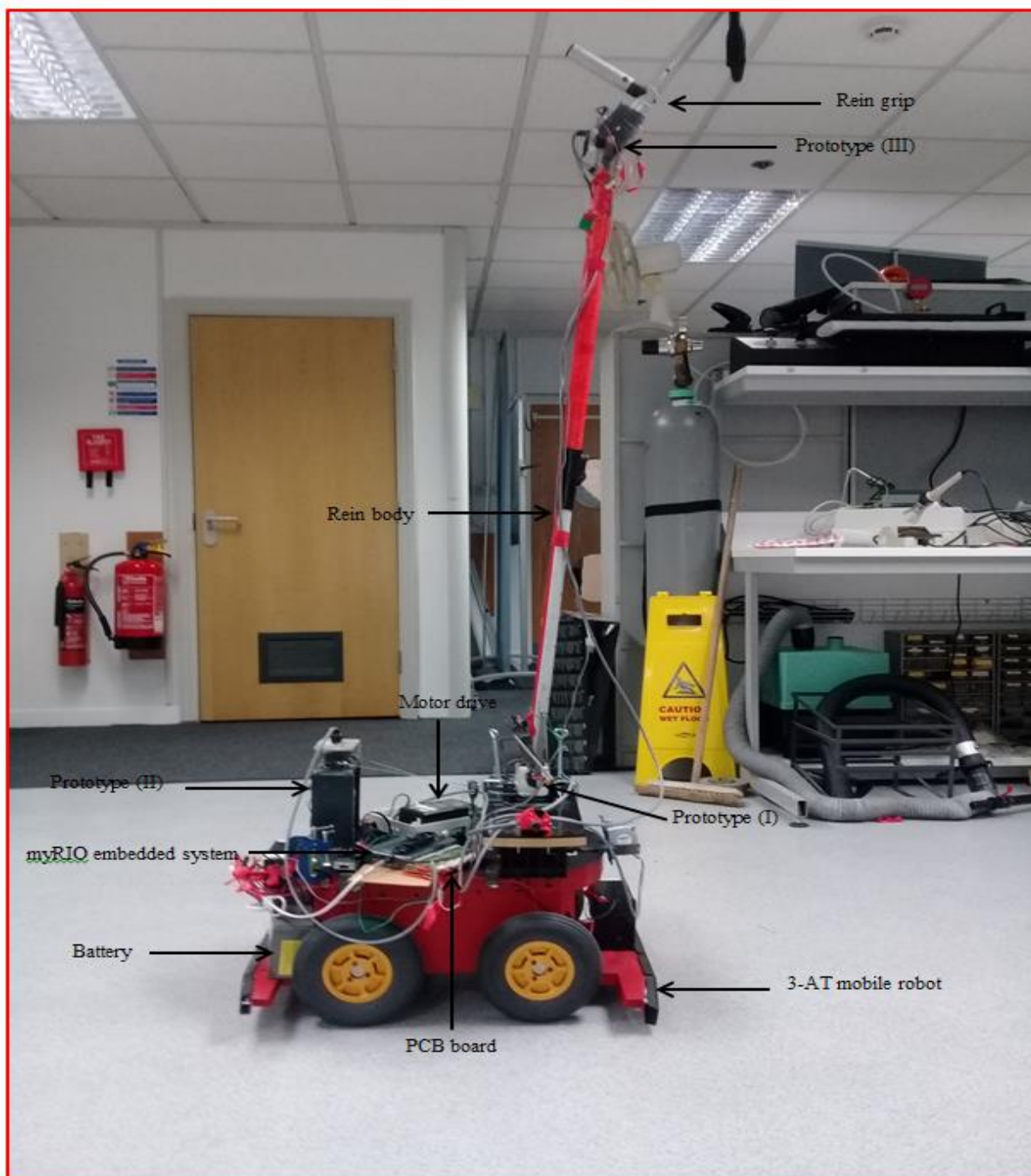
Figure (7.8) Real whole system structure.
