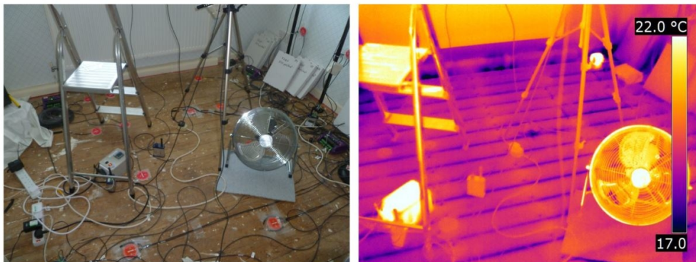
Figure 5, Infiltration through the ground floor
