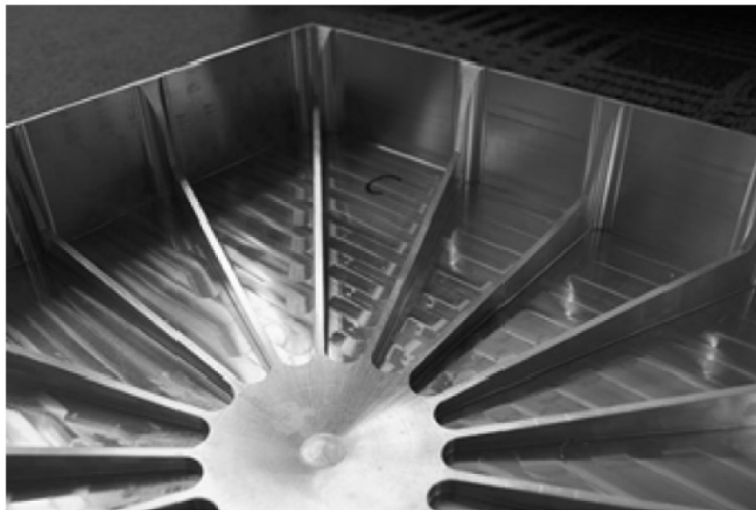
Figure 7. Detail of the floor stiffening ribs and wall buttresses in the pan preform.
