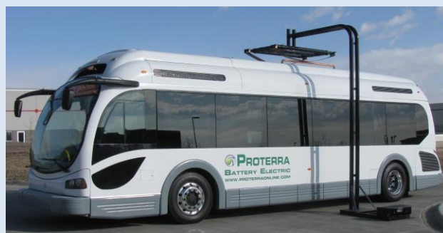
A Proterra zero-emission bus and charging station
