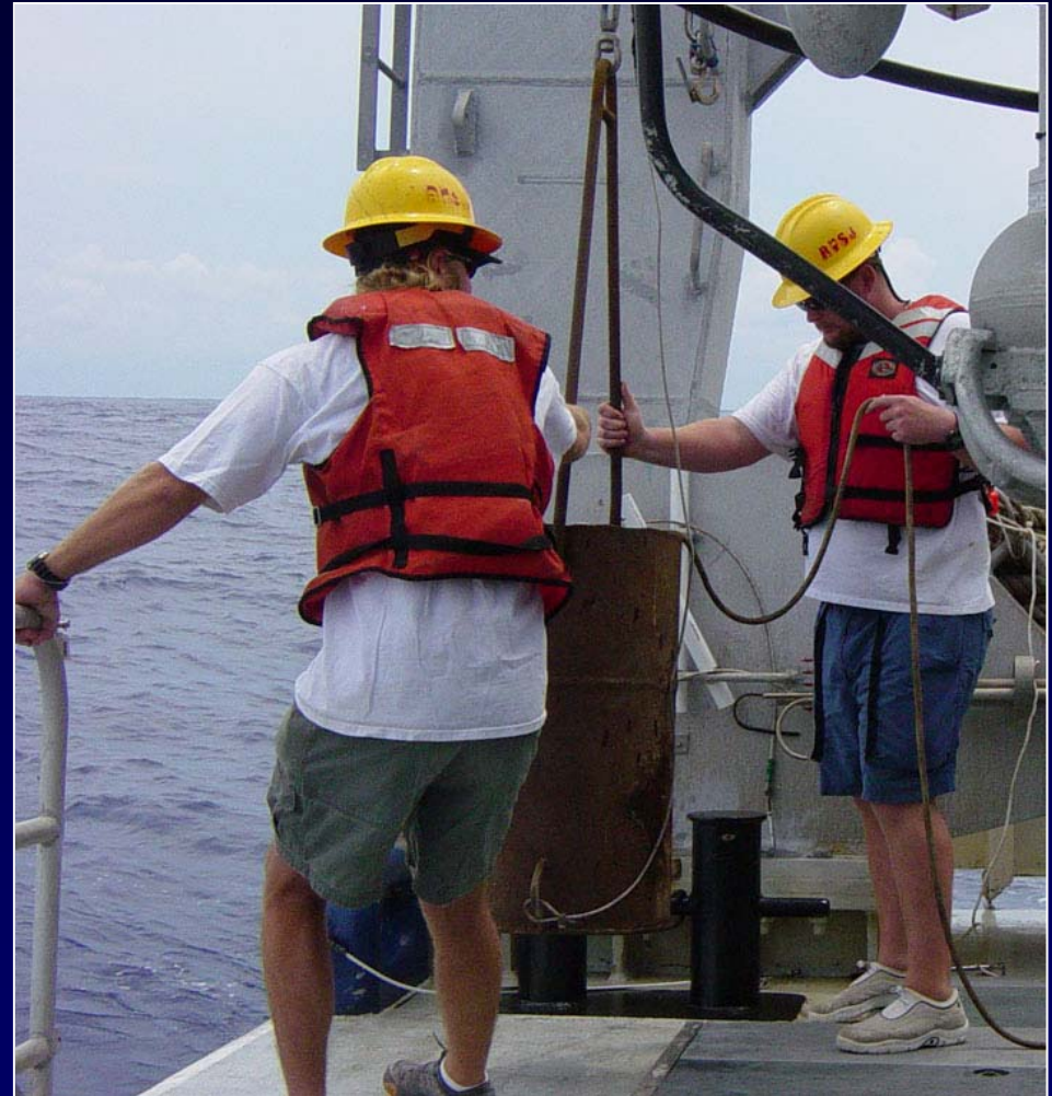
The pipe dredge is deployed from the ship's stern.
