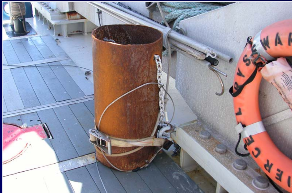
An inexpensive but nearly indestructible pipe dredge.
